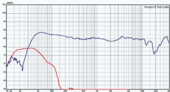
Graph 3. Nearfield response of port (red trace) and nearfield response of mid/bass driver, with far-field tweeter.
